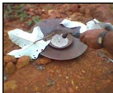
Figure 6: Burning of amalgam for extraction of gold.
