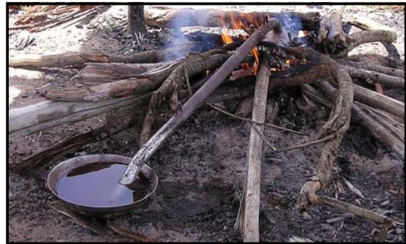
**Figure 8: Retort heated on fire with kuoy to recover mercury.**
