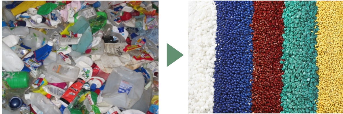
Figure 14: Recycling PE / PP (left) into possible products after the recycling process (right)
