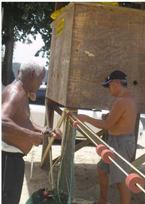
Trinidad net makers prepare gillnets for the surface-set gillnet fishery. Nets used in this fishery are made of twisted nylon twine with a 9.35 cm mesh size. © Scott A. Eckert - WIDECAST.
