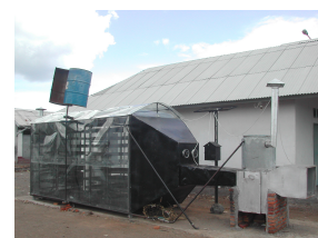
Wind power fish dryer prototype under test in Tanjung Luar, West Nusa Tenggara.
