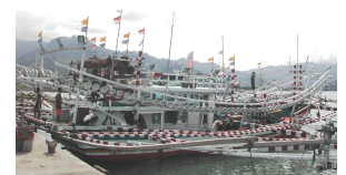
A liftnet boat docked in Bungus, Padang, North Sumatra with its 140 lamps.
