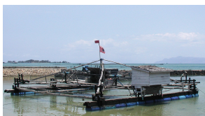
First generation design of mobile liftnets mounted on rafts and towed to the fishing ground.
