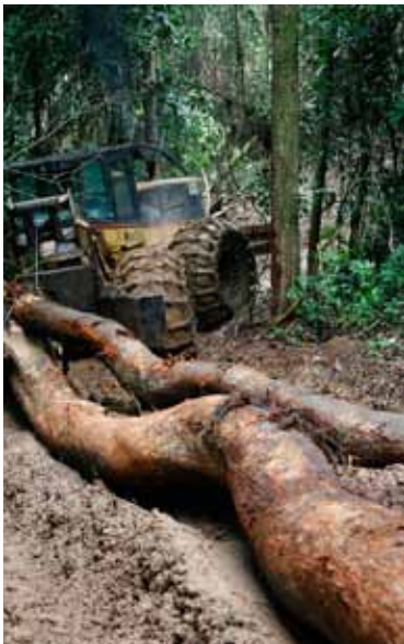
A "track skidder" at work in the forest in Western Ghana. The skidder pulls the tree from the production site to the road where it will be loaded onto trucks.
