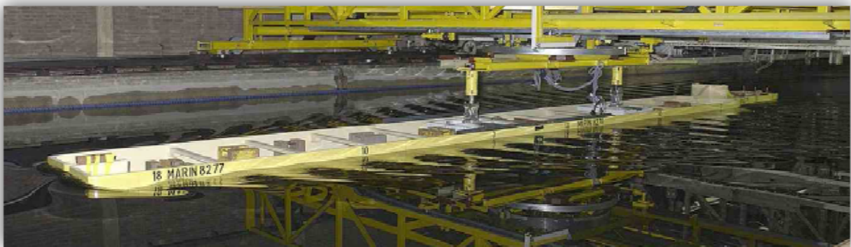
Figure 7.2 Model tests of a push train – an example of good wave system optimised by Contemporary Computational Fluid Dynamics (CFD) (Source: MARIN)
