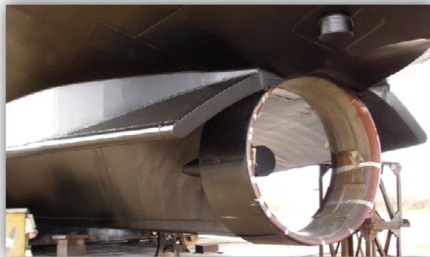
Figure 7.5 Special attention should be paid to tunnel and skirt design to enable better water inflow to the propeller
