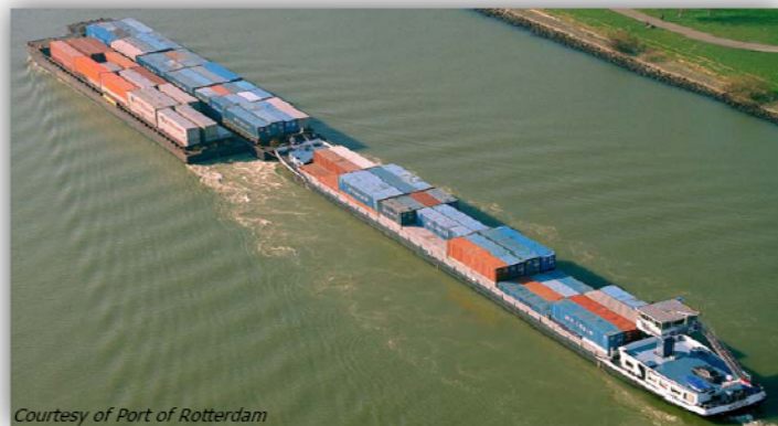
Figure 5.3 Coupling train on the Rhine with a typical container ship of 4 \times 4 \times 13 = 208 TEUs
