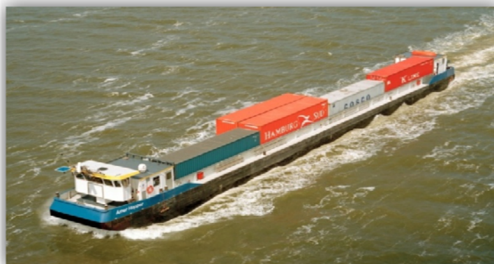
Figure 5.4 Small container vessel “Amer Hopper” - 86 \times 7.03 \times 2.86 m (Source: Mercurius)
