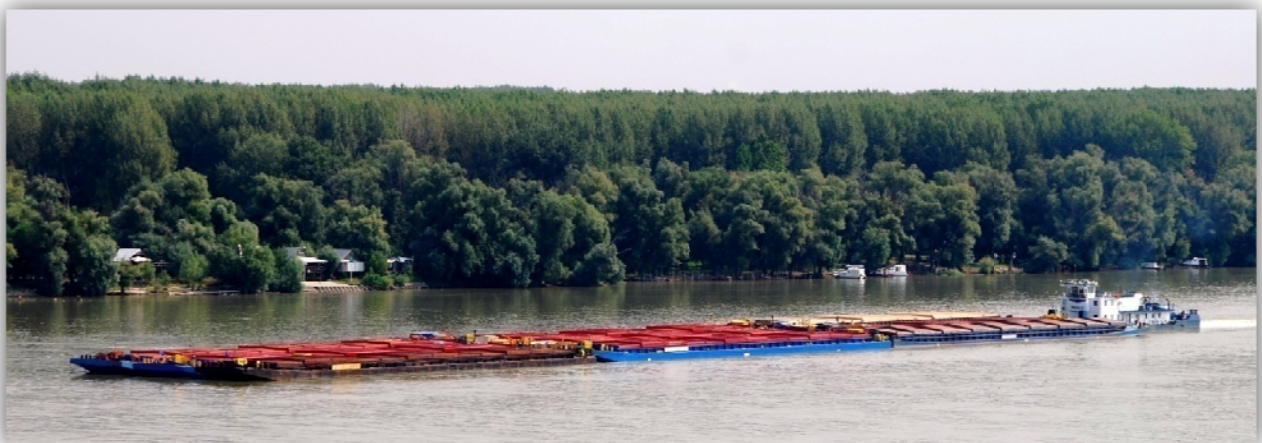
Figure 5.13 Pushing train consisting of 9 Europe II barges (about 260 x 34.2 m)
