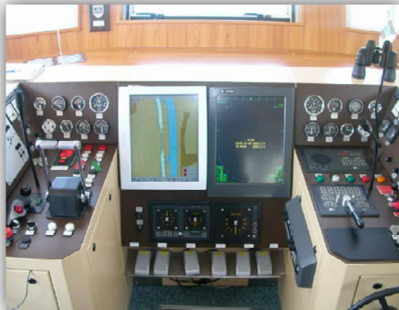
Figure 7.25 Bridge computerization on river vessel (Source: Witteveen-Bos)
