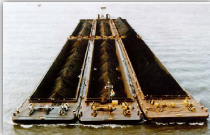
Figure 5.12 Pushing train consisting of 6 Europe II barges - about 190x34.2 m, up to 16,000 tdw depending on the draught (Source: CREATING WP5)
