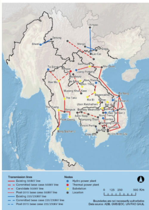
Map of GMS Planned and Current Transmission Line Interconnections. Credit: GMS Atlas of the Environment, October 2013 < www.gms-eoc.org >
