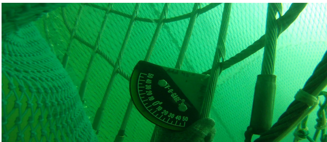
Figure 36 A perfect LR shape results in a perfect angle- 45°
