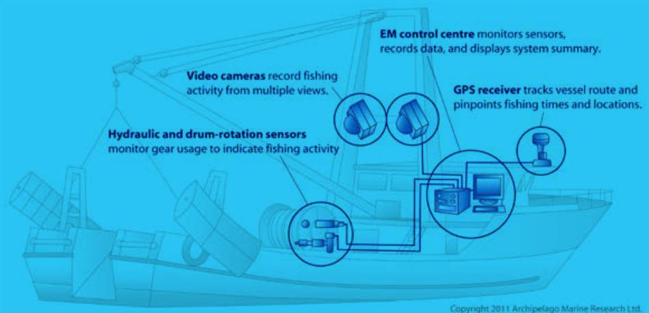
Figure 1. Diagram of a remote electronic monitoring system (REM) installed on a fishing vessel (Courtesy of Archipelago Marine Research Ltd.).
