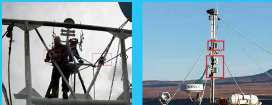
Figure 2. Cameras installed on fishing vessels
