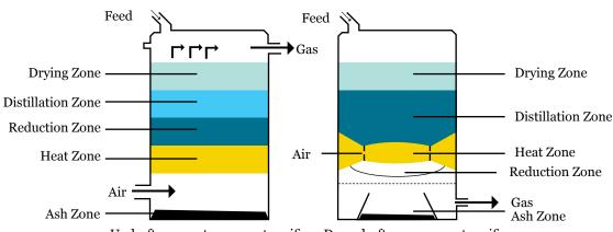
Updraft or counter-current gasifier Downdraft or co-current gasifier
