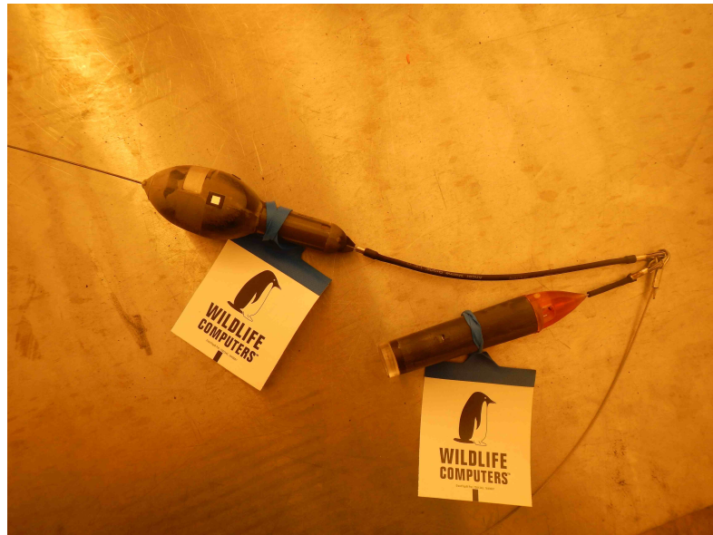
Figure 4: mrPAT and pop off archival satellite tag attachment design for trial on Greenland sharks in Grise Fjord.
