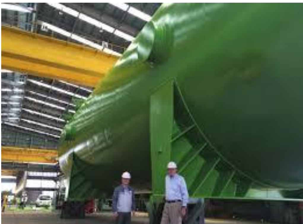
Figure 8: Example of Type C Tank (for TOTE container ship)
