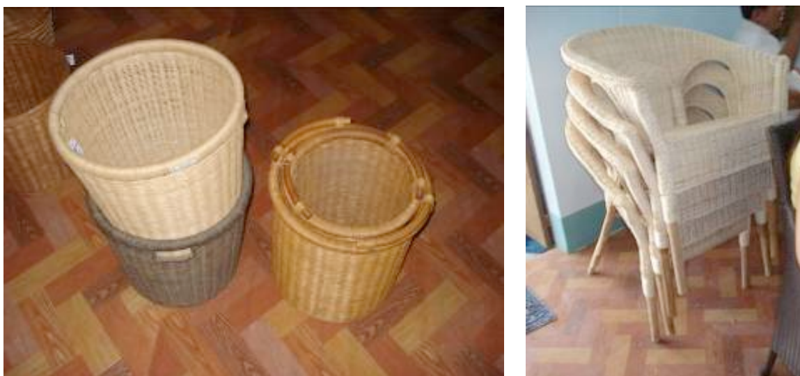
Figure 24. Ways to save transportation room in packaging
