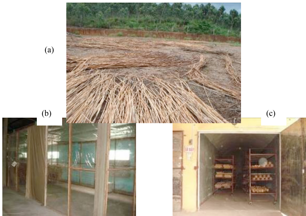
Figure 11. Natural drying (a), drying chamber using secondary solar radiation (b), drying room (c)
