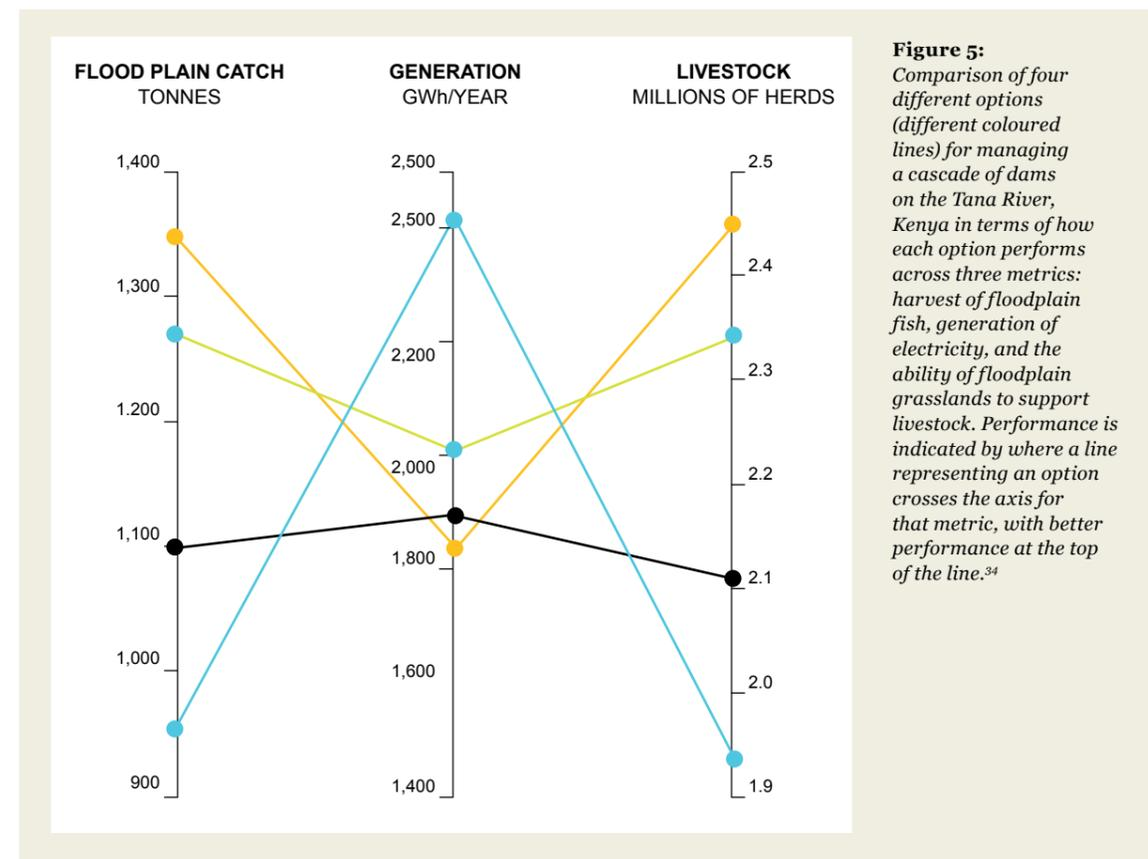
**Figure 5:** Comparison of four different options (different coloured lines) for managing a cascade of dams on the Tana River, Kenya in terms of how each option performs across three metrics: harvest of floodplain fish, generation of electricity, and the ability of floodplain grasslands to support livestock. Performance is indicated by where a line crosses the axis for that metric, with better performance at the top of the line.<sup>34</sup>
