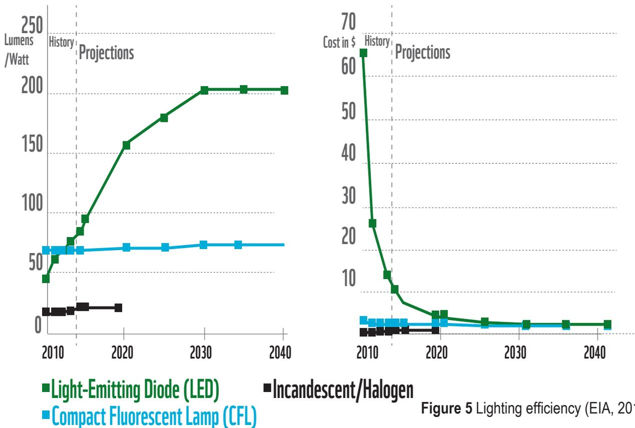
Figure 5 Lighting efficiency (EIA, 2014)
