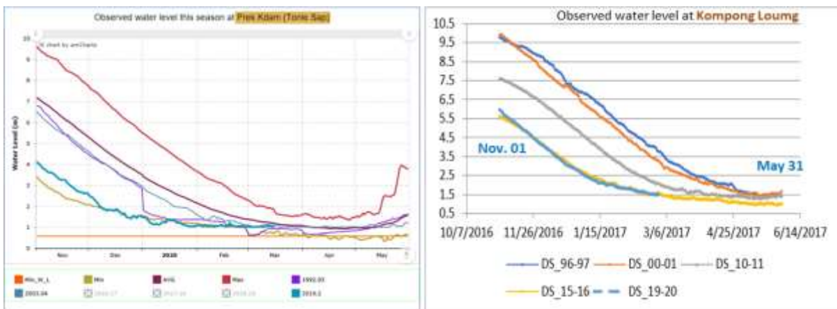
Figure 12. Water levels at Prekdam (left) and Kompong Luong (right) stations on the Tonle Sap River
